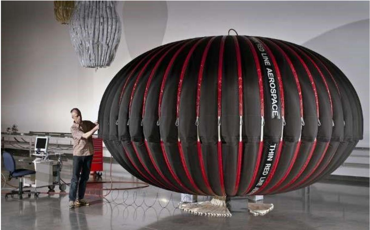
*Underwater compressed air energy storage (UWCAES) is a method for storing energy in the form of compressed air. In an UWCAES system, electrical energy is converted to and from compressed air using a series of air compressors or turbo-expanders.*
